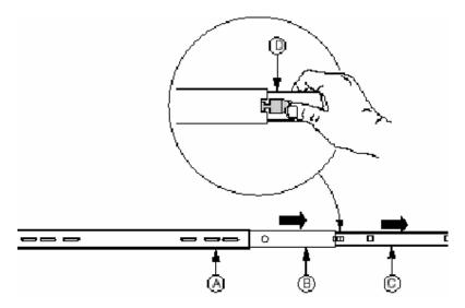
Figure 35: Removing the Rails
